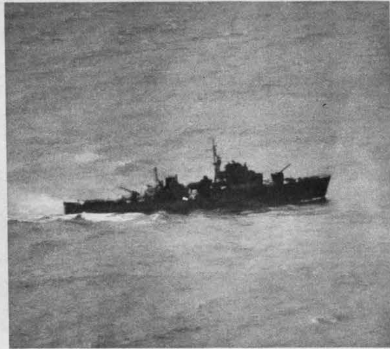
Most important PF is new Kaibokan 1, now being seen in numbers. Stack aft, straight raked bow, shielded forward gun are typically Jap.
